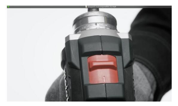
Before drilling, make sure of the following. The power tool is put in **gear one**
