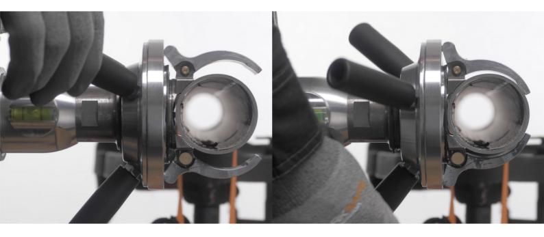
Extend the foldable handles, open the clamp, and tighten Snapdrill to the pipe.
