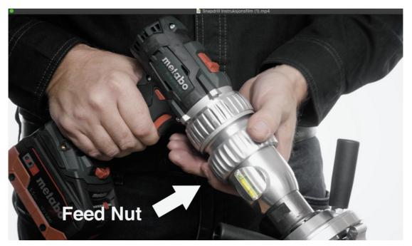
Tighten the feed nut. Pull the trigger and let the insert area come forward.
