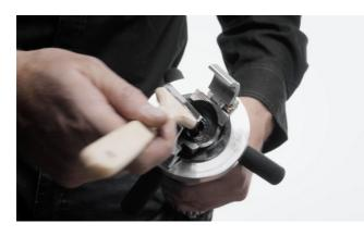
Regularly clean Snapdrill for metal shavings. Use a brush or a magnet. Do not use pressured air.
