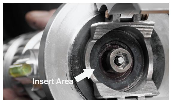
Snapdrill and the battery drill need to be connected in order to insert hole saws.
