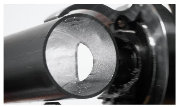
Once drilling is completed, do not yet return the hole saw, loosen the handles. First with two hands, then with one hand while holding the battery drill with the other. Remove Snapdrill from the pipe.
